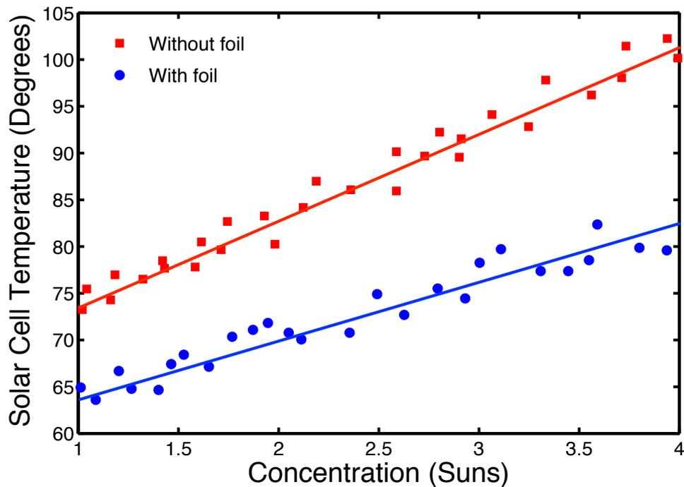
**Fig. 5** Solar Cell temperature measured versus concentration with and without Solar Bankers optical grating. The measurement was carried out in field, with an outside temperature  $T_{\text{ambient}}$  of  $45\text{ }^{\circ}\text{C}$ . The concentration of 1 Sun
