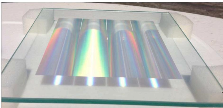
**Fig. 3 Picture of Solar Bankers' holographic grating. It consists of a micrometric-thick polymeric layer that separates light colors and concentrates only wavelengths suitable for PV conversion.**
