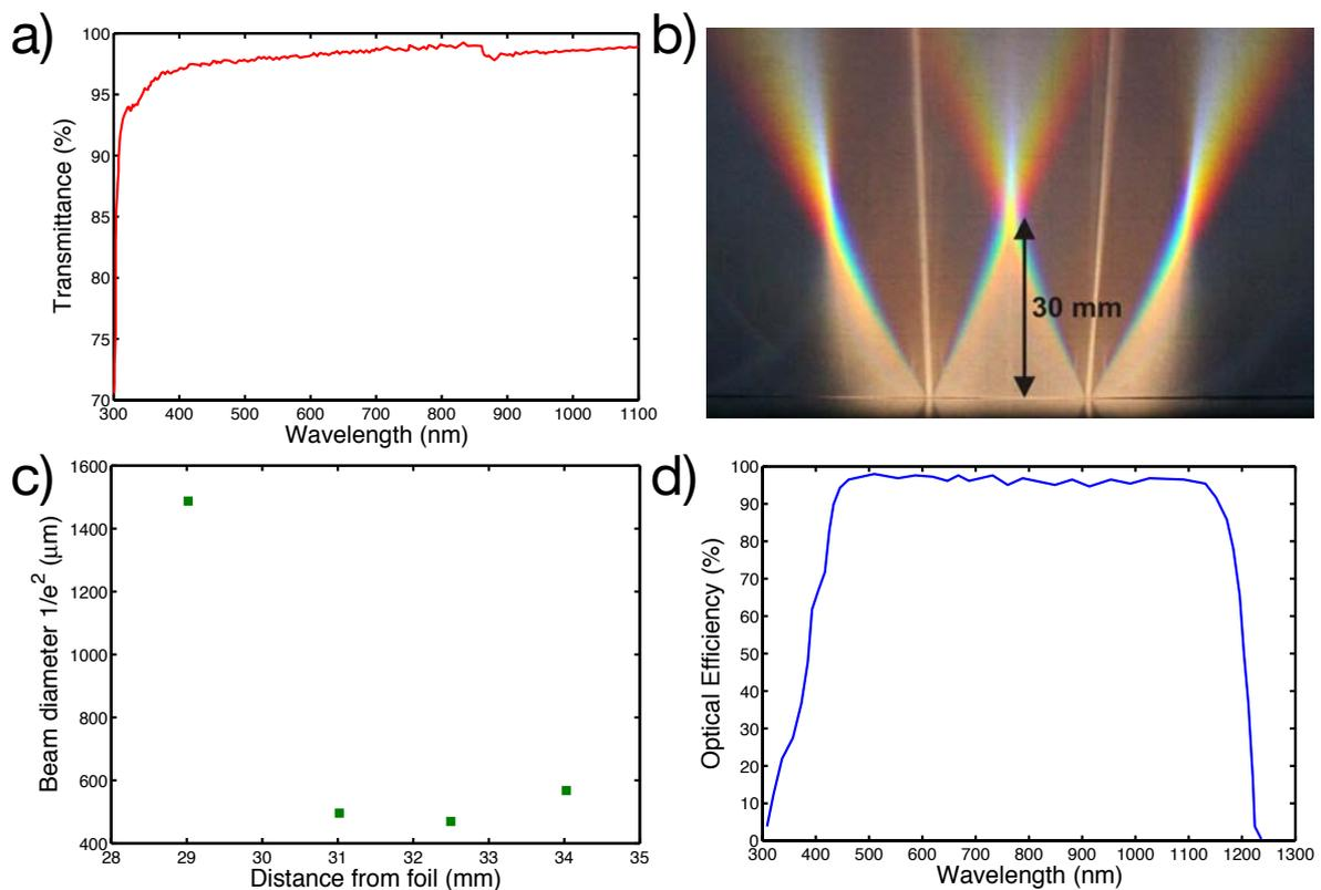
**Fig. 4** a) Transmittance of the optical grating measured in the spectral range 300-1100 nm; b) Picture of the light pattern transmitted by the optical film when illuminated with a white, halogen lamp; c) Diameter of the light beam
