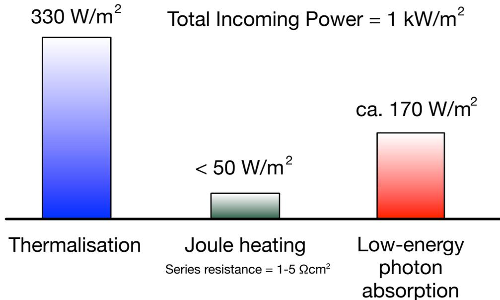
Fig. 1 Mechanisms of heat generation in solar cells and related energy contributions calculated for the ideal case of a 33%-efficient Silicon solar cell.
