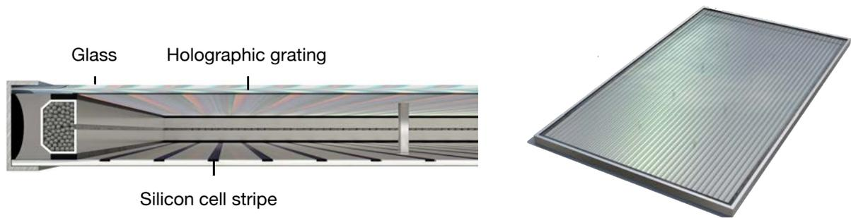
**Fig. 2 Representations of Solar Bankers' PV module, which is comprised of a glass, a holographic grating and high-efficiency, back-contact Si solar cells. The thickness of the module is 4.6 cm and the internal volume is filled with nitrogen to prevent polymer degradation.**
